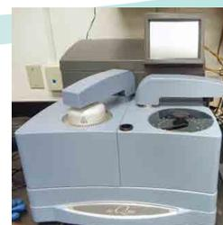
*Emerald's R&D team uses a wide variety of analytical instruments to evaluate plasticizer performance in applications such as adhesives, including a 90° peel fixture to evaluate quick stick (top) and a DSC to determine Tg (bottom).*
