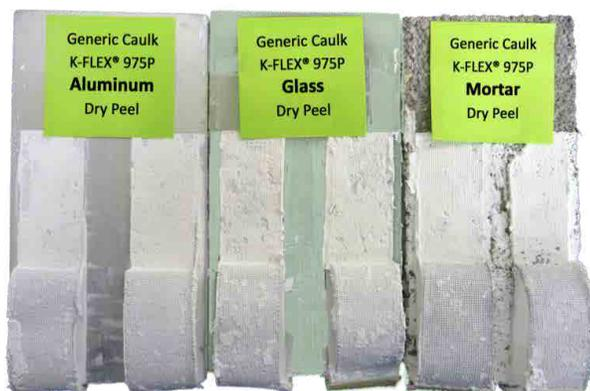
*K-FLEX® 975P provided excellent adhesion-in-peel when tested in an ASTM C920 latex caulk over aluminum, glass, and mortar substrates.*
